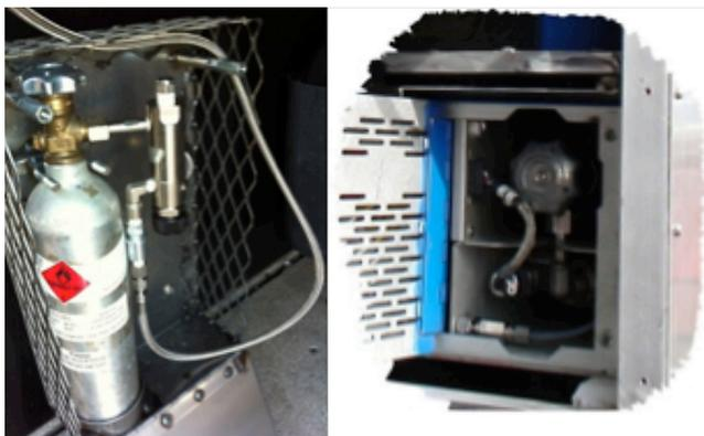
Figure 2. The Flammable FID Fuel Cylinder is enclosed within PEMS enclosures as required by the DOT-SP. Note the EFPV installed on the unit in the left photo
